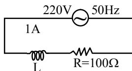
For the full to be operated at its rated value the rms current through it should be 1A
